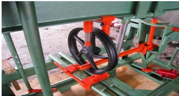
*Gambar 2.21. Press Pelek Racing otomatis*
