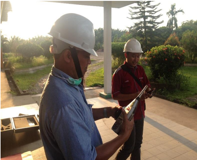
Proses Kalibrasi alat Sound Level Meter
