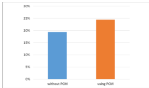
Fig.16 Comparison of desalination equipment efficiency without PCM and using PCM
