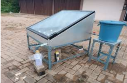
Fig.6 Seawater desalination equipment
