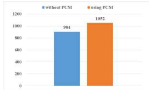
Fig.15 Comparison of the average amount of fresh water produced from 3 experiments without PCM and 3 experiments using PCM
