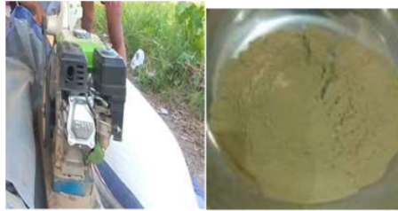
Fig.3 Milling process Rija-rija fiber is micron-sized and pre-treated with an acid solution.
