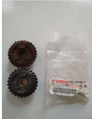
Gambar 1. Roda gigi mesin speed yamaha enduro 15PK
